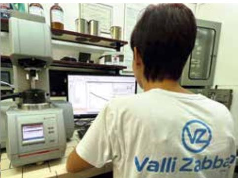
Indagini sui bitumi: test DSR Dynamic Shear Rheometer
