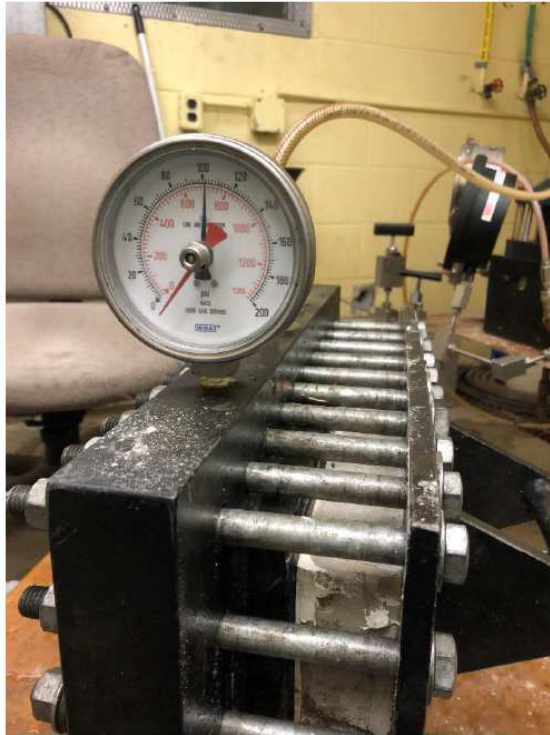
Sample sustained 100 psi later water head pressure.
