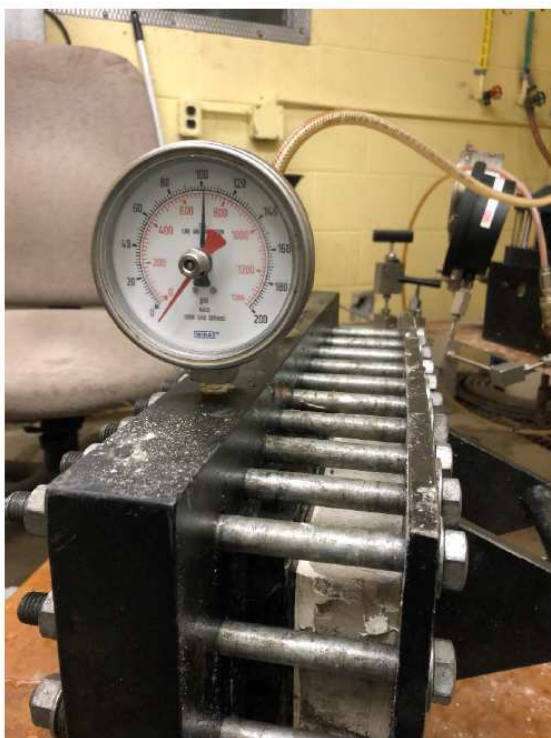
Sample sustained 100 psi later water head pressure.
