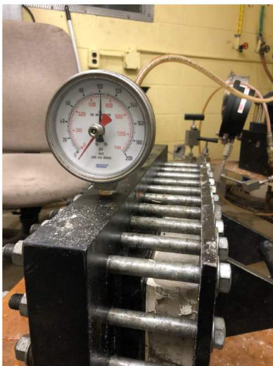
Sample sustained 100 psi later water head pressure.
